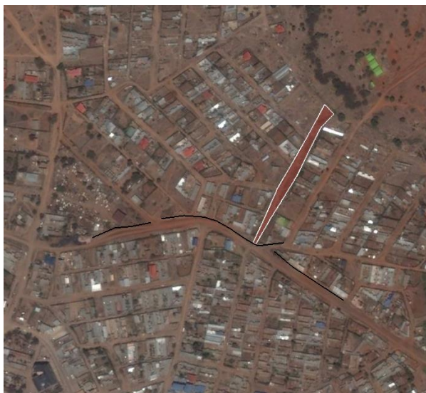
Figure 21 Options: red with white outline, gully rehabilitation; black line: storm drain with perforated bottom and trees
