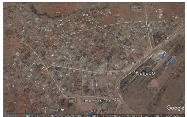
Figure 4 Flow direction of road drainage along major roads.
